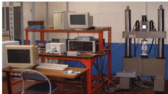
Fig. 4. Experimental apparatus for dynamic test on MTS machine (ISMEP, Paris).
